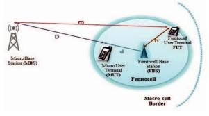
Fig. 2. Example of spectrum sharing between macro and femto cell.
