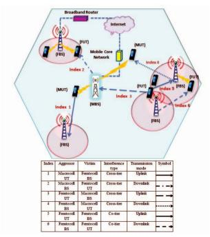
Fig. 1. Interference scenarios in heterogonous networks.
